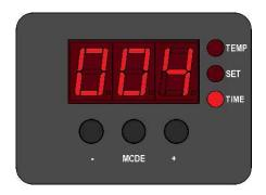
The timer will count down and audibly signal you to lift the heat platen into the UP position when the press cycle is complete. The time will automatically re-set and you are ready to continue with the next application.
