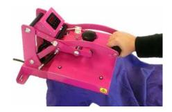
Lower and lock the heat platen into the press position. The automatic timing process will start.
