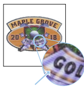
Minimum size floating and space between floating elements: 0.040" / 1mm
