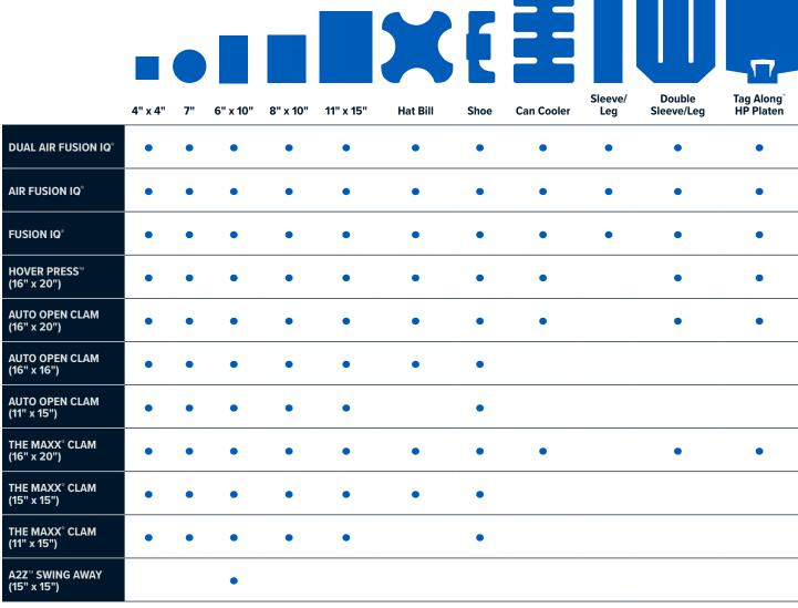
All Quick Change Heat Press Platens are only compatible with heat presses manufactured after 2014. Custom platens are available.
