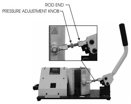
Adjust the pressure by turning the knob clockwise to increase pressure and counter clockwise to decrease the pressure.
