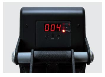
Once you have adjusted the temperature, press the Mode Select button again to advance to Time Mode.
